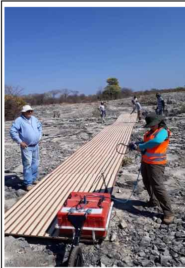
Figure 1 - A simple methodology to perform GPR surveys on very rough terrains.
