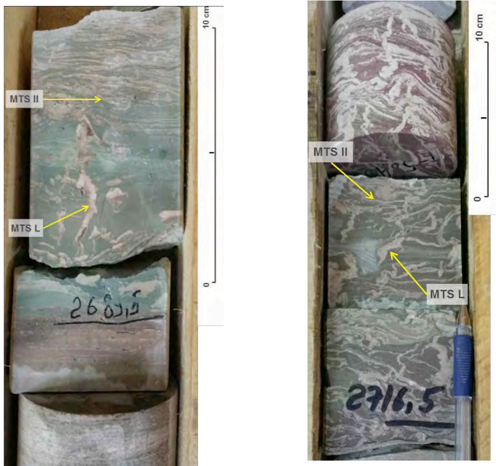
Fig. 1. Example of MT structures in Riphean dolomite of West Siberia MT II – subparallel to layering, MTL – perpendicular to layering
